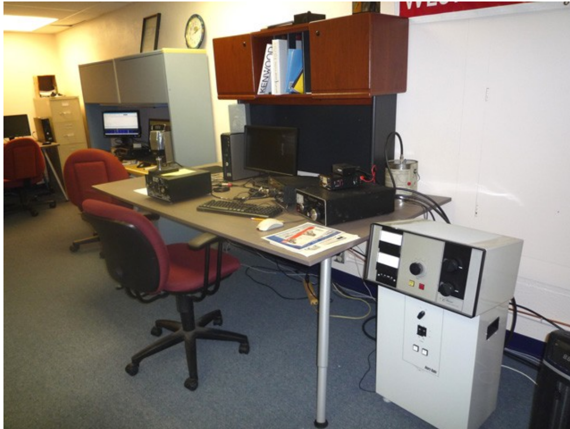
HF Position 2 (note Henry 2K amplifier)
