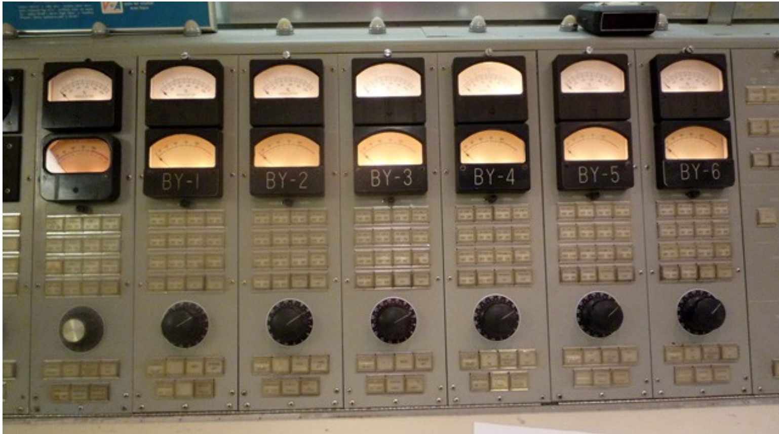
Meters: % modulation (upper), VU (lower)
