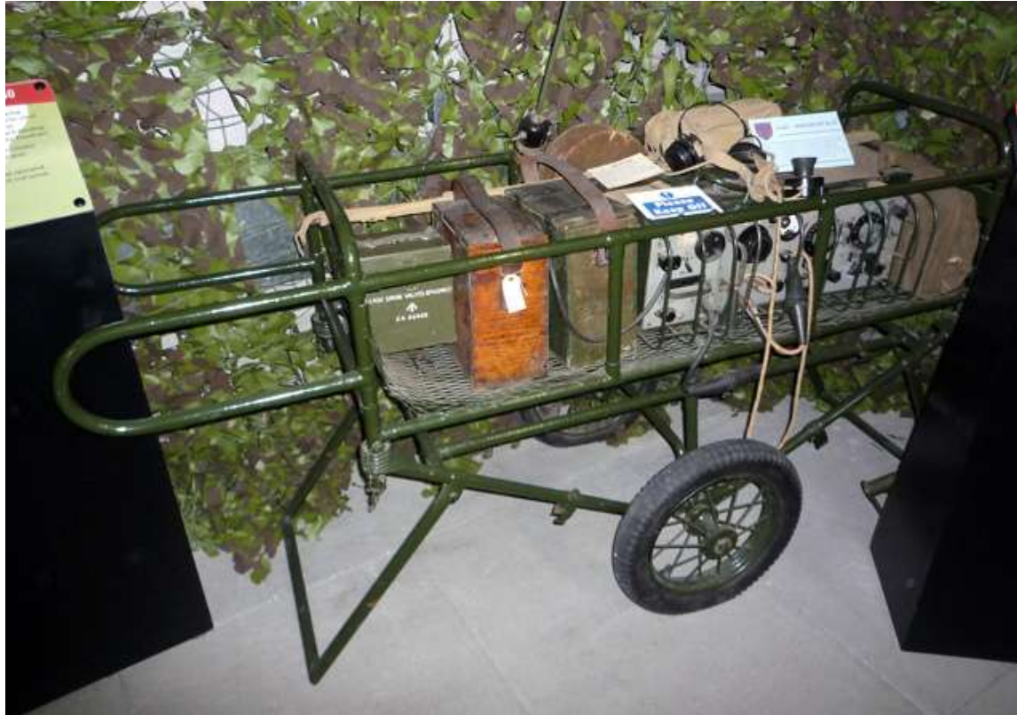
The “wireless pram” carried a No. 22 set (2W, 2 – 8 MHz) with vibrator PSU and batteries. A RSigs radio operator earned the George Medal pushing one of these beasts around between landing zones under withering German fire. (He survived!) Note antenna on top.
