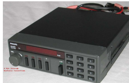
MX290 series, 1982-89. VHF/UHF, 5-25W, 80 ch., 1st synthesised mobile
