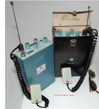
Bantam: 1965 25-68, 68-174 MHz 1W, AM/FM Weight ≈ 2 kg
