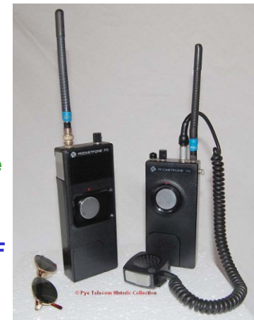
Pocketfone PF2 PTL's 1 st complete HT line, 68-174 & 450-470MHz 1W VHF, 0.1W UHF Weight ≈ 600g
