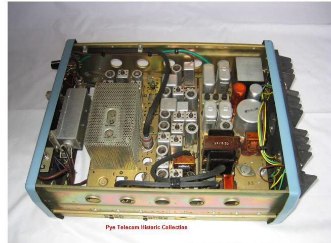
Ranger Series (PTC2001/8001): 1955 – 1963; various configurations PTC8001 was 1st solid-state mobile 25 – 174 MHz; 9 ranges produced 5-25W AM, 10-25W FM Separate TX, RX & squelch PSU strips for enhanced configurability 20-120 kHz channel spacing for UK & international markets (incl. Canada)
