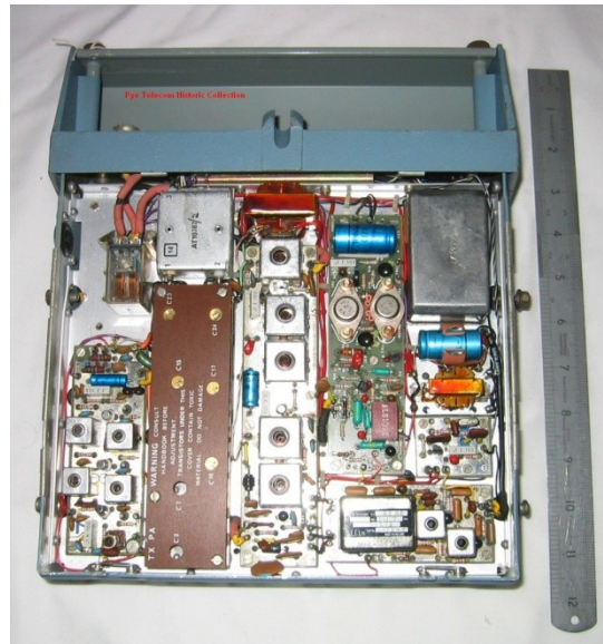
Cambridge, showing solid-state RX modules: 1961-1970 25-174 & 440-470 MHz 7-10W AM, 25W FM, 5W UHF
