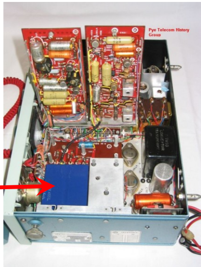
Cambridge, showing solid-state RX modules: 1961-1970 25-174 & 440-470 MHz 7-10W AM, 25W FM, 5W UHF
