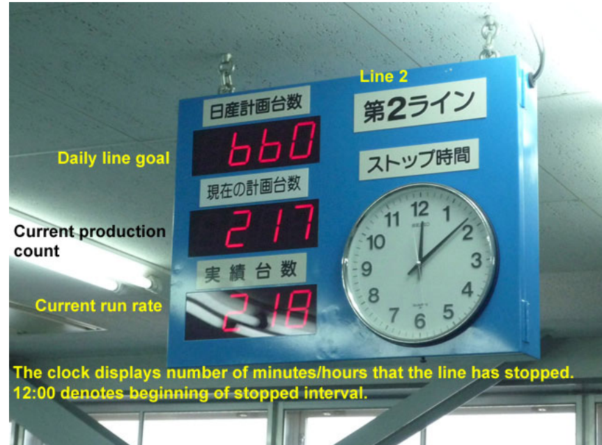
Line status display.
