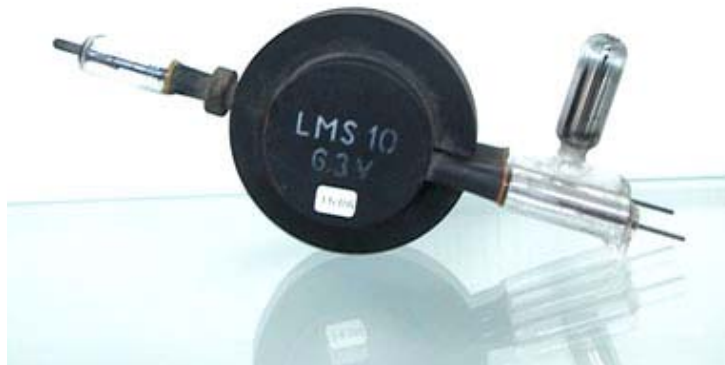
German LMS 10 cavity magnetron: 15 kW peak pulse at 3.3 GHz
