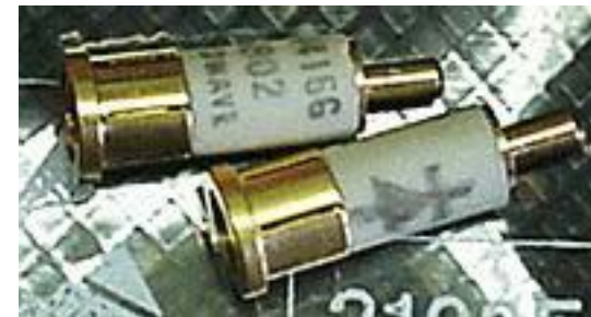
1N416 Si Mixer Diodes: used in US and British radar receivers (NF 6 – 7 dB)
