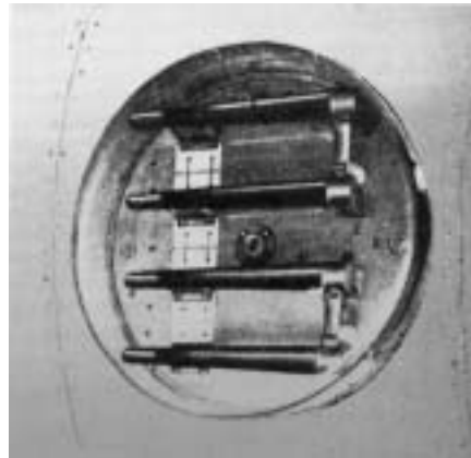
4-element polyrod antenna, downward- looking & rotating at 400 rpm.
