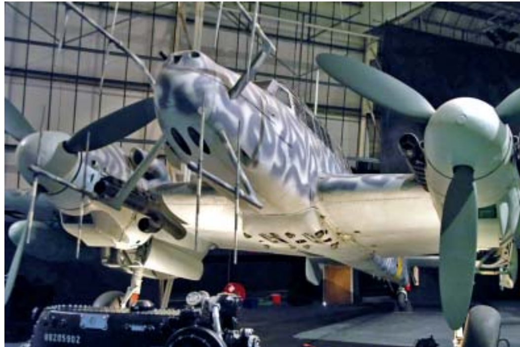
Messerschmitt Bf 110 G-4 in the RAF museum at Hendon, with second-generation FuG 220 (Lichtenstein SN-2) and nose-mounted antenna array. These large antenna structures had significant drag, and could lop as much as 50 km/h off the top speed of an aircraft.
