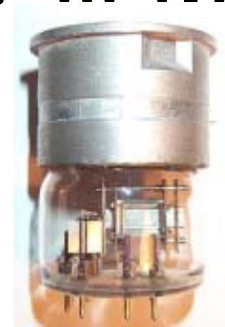
Telefunken LG2 Dual Diode Würzburg RX Mixer (NF 16 dB)
