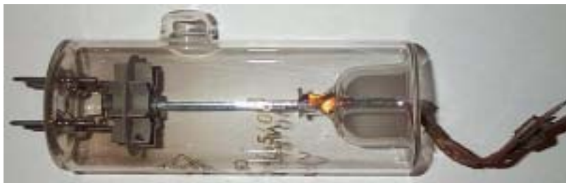
Telefunken LS180 Power Triode: Würzburg TX PA Peak pulse output 7 – 11 kW
