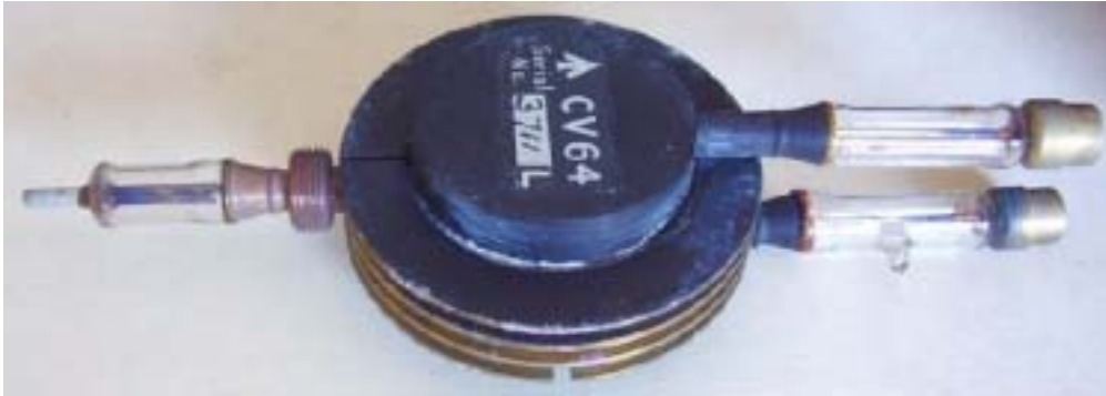
British CV64 cavity magnetron: 40 kW peak pulse at 3.3 GHz
