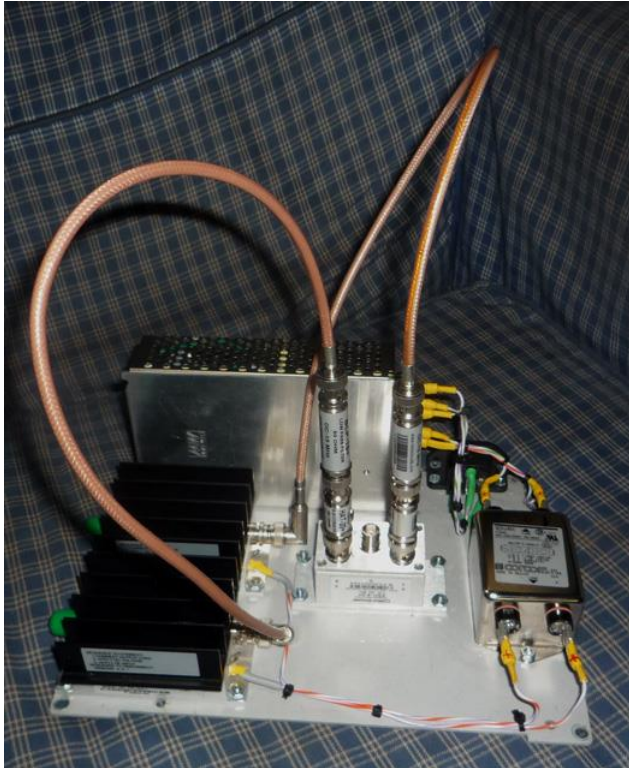
2-SIGNAL IMD TEST FIXTURE
