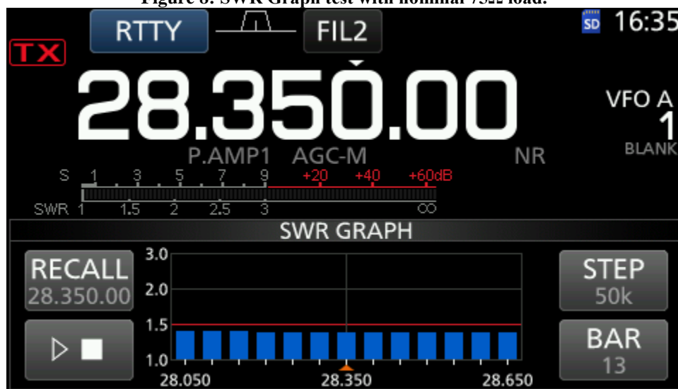
Figure 8: SWR Graph test with nominal 75Ω load.
