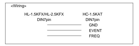
FREQ data: Freq. data signal is sent to tuner.
