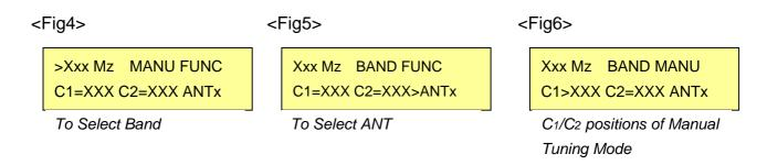
" > " mark is displayed at this time to urge the setting of Band, Ant, and  $C_1/C_2$  respectively.
