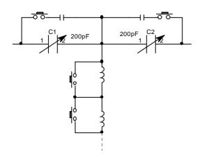
C1, C2 = 200 pF max, 3 kV L = Switched by relays Fixed C = Mica caps., 3 kV
