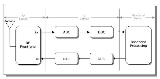
Figure 1: Block diagram of a generic digital transceiver
