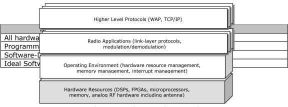
Figure 2: Software Architecture of SDR
