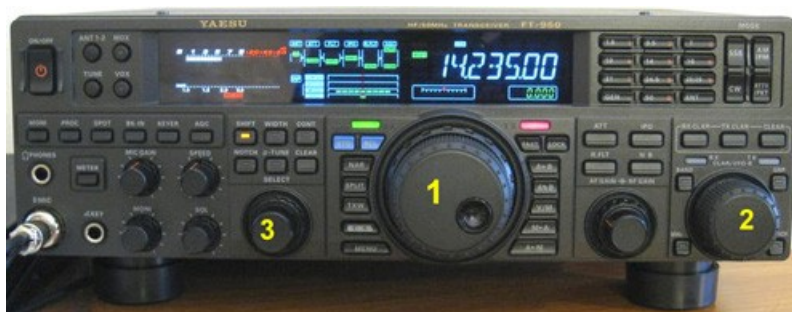
Figure 3: Yaesu FT-950 showing main controls.
